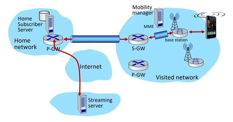
tunneling via GTP (GPRS tunneling protocol): mobile's datagram to streaming server encapsulated using GTP inside UDP, inside datagram
