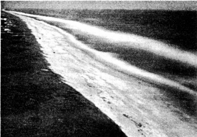
Figure 7-5 Oblique video images of the nearshore at the Field Research Facility, Duck, North Carolina. (a) A snapshot shows the instantaneous patterns of wave breaking that are suggestive of the beach bathymetry, particularly the presence of an offshore bar. (b) A 10-minute time exposure yields a white band in the offshore from many occurrences of wave breaking, showing the outlines of the bar and a zone of wave dissipation due to swash on the beach face. [Used with permission of American Geophysical Union, from T. C. Lippmann and R. A. Holman, Quantification of Sand Bar Morphology: A Video Technique Based on Wave Dissipation, Journal of Geophysical Research 94, p. 996. Copyright © 1989 American Geophysical Union.]
