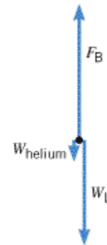
(b) Free-body diagram of the airship
