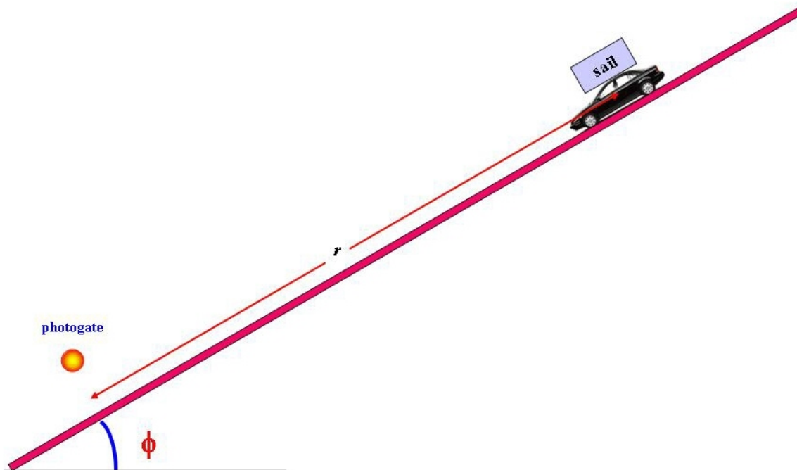
FIG. 2: Experimental set-up for measuring kinetic energy on an inclined plane.
