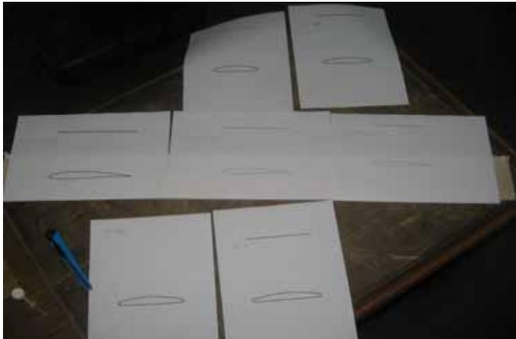
3. Printed sections are placed to be cut.
