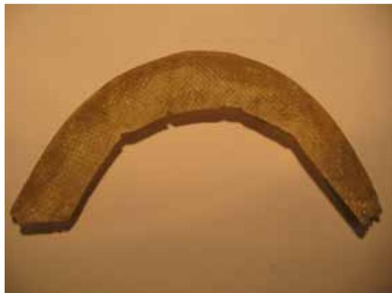
**Figure 6.16** First trial of fiber glass leading edge
