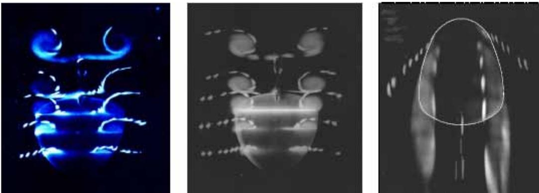
Figure 2.4 Wingtip Vortices, ziminv1.00 Wing,  $Re \approx 70,000$ ,  $\alpha = 15^\circ$
