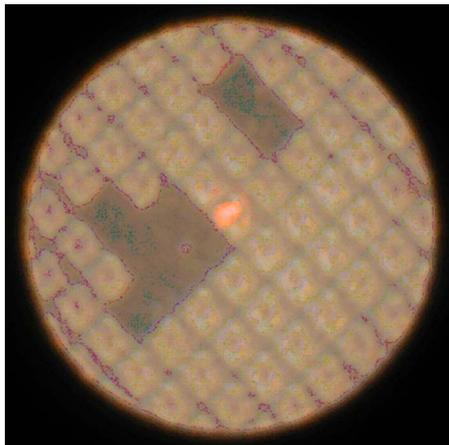
FIG. 1. (Color online) DMD surface viewed through a 400 mm lens and 40 $\times$  eyepiece. Dark areas are mirrors damaged by high laser powers. Light areas are undamaged mirrors. The red spot is the HeNe laser reflecting off a single mirror.
