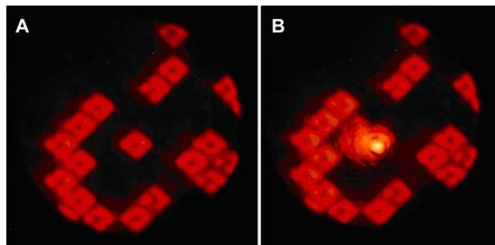
FIG. 3. (Color online) Images taken through the ocular shown in Fig. 2. (a) Micromirrors at the edges of the DMD active area illuminated with red light. (b) 633 nm laser focused on a single micromirror. Dark areas are micromirrors in the off position.
