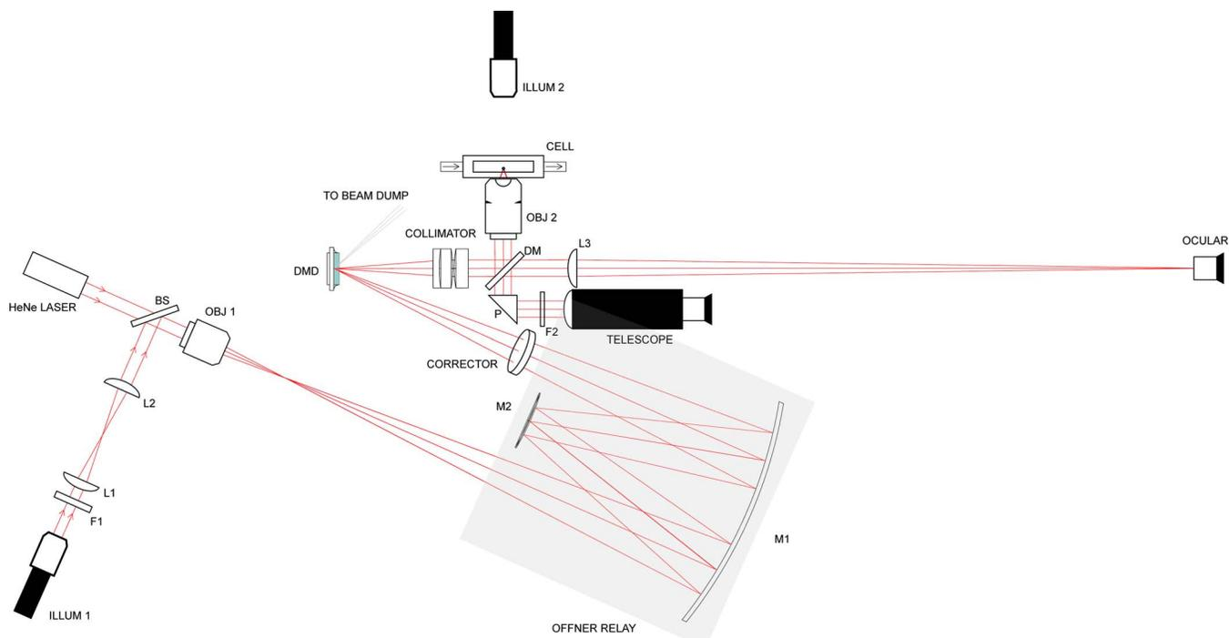
FIG. 2. (Color online) A system incorporating the DMD for creation and control of a single trap.
