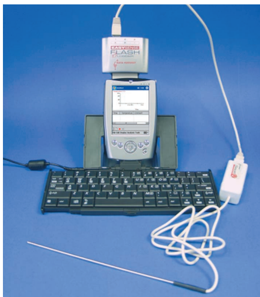
Figure 1. Project Numina hardware. UNCW students use a pocket PC, such as this Dell Axim X5, with temperature probe and Compact-Flash data logger, in science labs.
