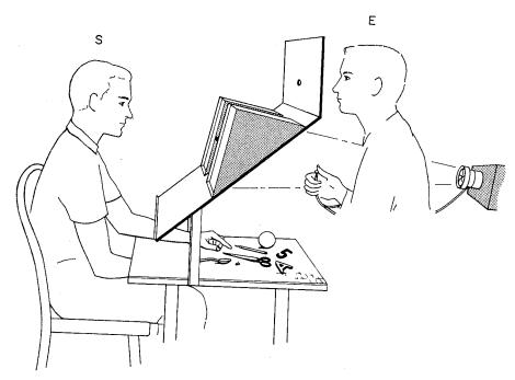
Testing apparatus: Slanting shield on table prevents subject from seeing test items on table, his hands, or the examiner. It contains ground glass viewing screen for back projection of  $2\times 2$  slides, and also serves to hold cards or other test items set before subject in free view. Examiner flashes slides when subject's gaze is seen to be properly centred on designated fixation point. A second examiner beside subject records trials and subject's reactions.
