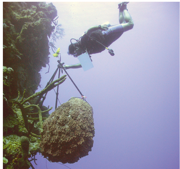
A diver positions an acoustic Doppler velocimeter over a Caribbean giant barrel sponge Xestospongia muta to measure the velocity of seawater pumped by the sponge.
