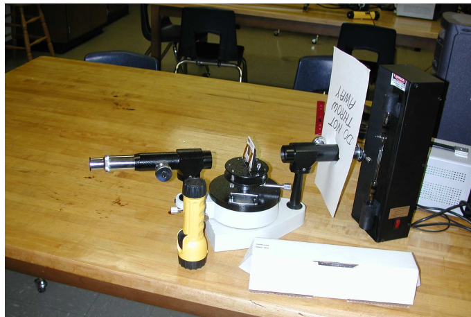
Figure 1: Experimental setup. In the foreground is a flashlight, behind which is the spectrometer. To the right of the spectrometer is the power supply with the hydrogen discharge tube mounted across its high voltage connectors.
