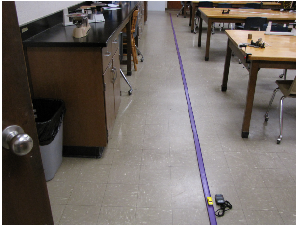
Figure 1: The equipment used in the experiment comprises timers, a hotwheels car, and 17 hotwheels tracks.
