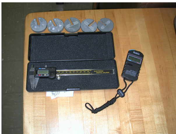
Figure 3: Additional equipment used in the experiment includes vernier calipers, five 100 gram masses, and a stop watch.
