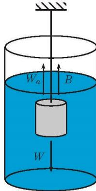
Figure 1: Archimedes Principle.
