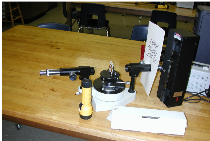
Figure 1: Experimental setup. In the foreground is a flashlight, behind which is the spectrometer. To the right of the spectrometer is the power supply with the helium discharge tube mounted across its high voltage connectors.
