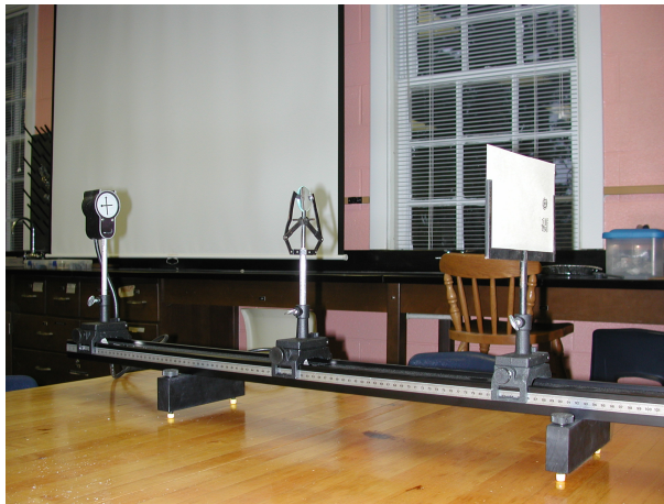
Figure 2: The optical bench. From left to right is the object, which consists of a light source and template, the converging lens, and a screen on which the image is projected.
