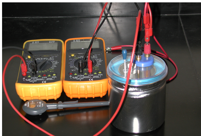
Figure 1: Experimental arrangement. The equipment used in this experiment includes a calorimeter, voltmeter, and ammeter. The resistor is located in a cup within the calorimeter.
