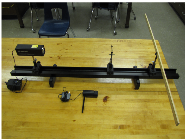
Figure 2: Positioned on the optical bench is the laser, the diffraction grating, and meter stick used for displaying the diffraction pattern. In the foreground is the LED point source used for producing the white light in the second part of the experiment.
