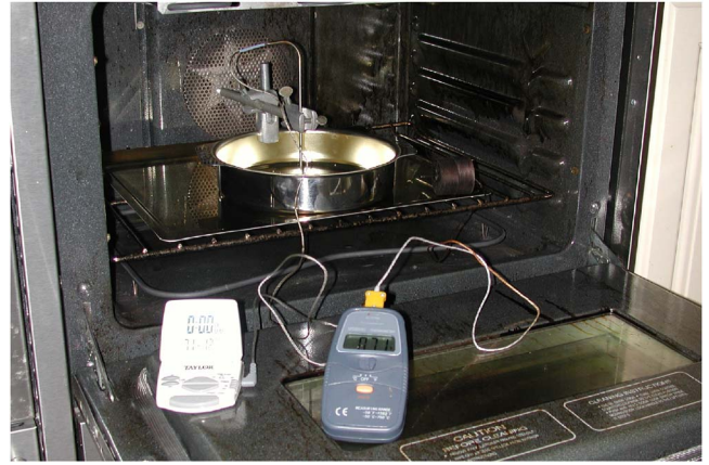
Fig. 1. The oven, baking pan, and two thermocouple sensors and temperature measuring instruments. One sensor monitors the internal temperature of the cake, and the other the temperature of the oven.
