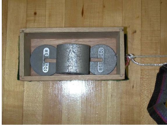
FIG. 2: Box and Weights. The 500-gram and two 100-gram masses are placed in the box as shown.
