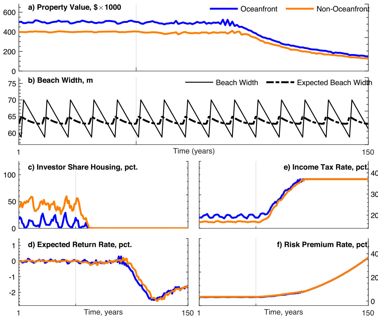
Fig. 3 | Baseline model scenario. The baseline case assumes that SLR begins at t=50 (marked by a vertical gray line) and continues throughout the remaining periods. Beach nourishment is subsidized at 90% of the cost. Outside property prices are constant, and agent flux is turned on (relatively high-income agents are able to enter to exploit arbitrage opportunities with outside markets). Depicts
