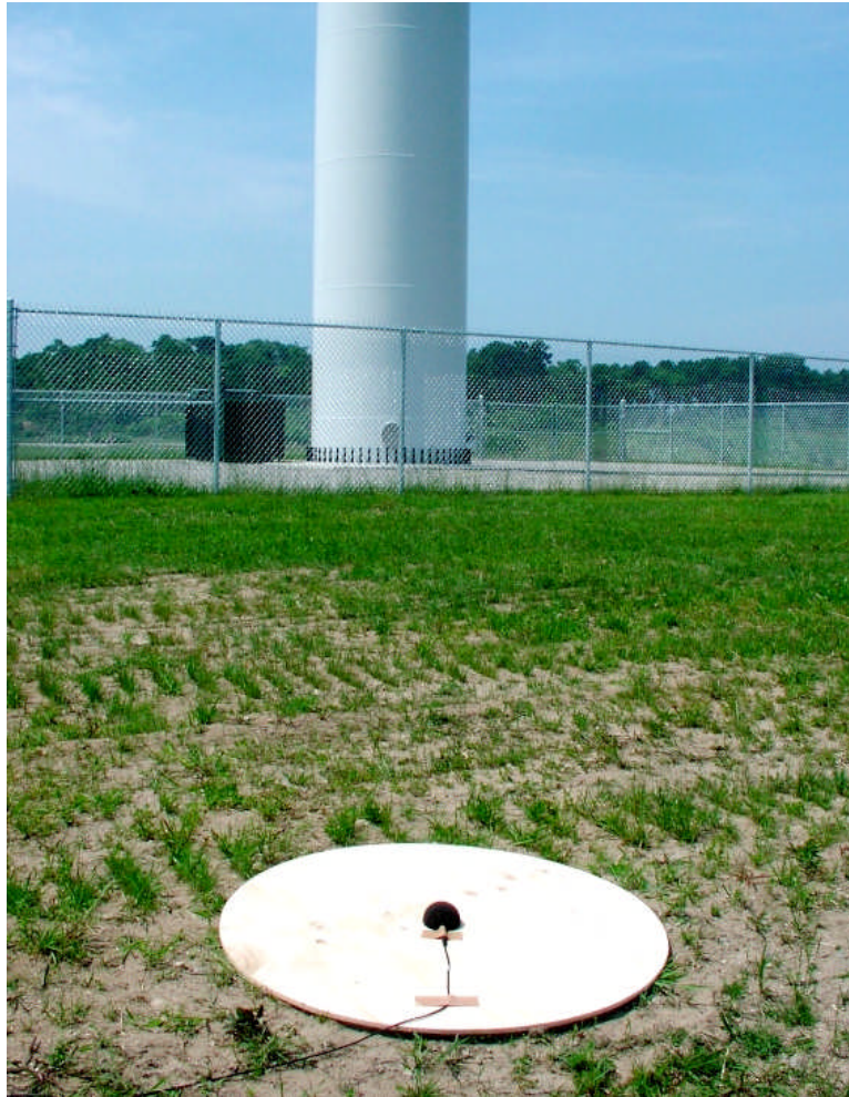
Figure 11 Photo of Reference Ground-plane Microphone and Wind-1 Turbine
