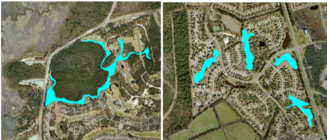
Figure 9: Site 3, a natural pond and Sites 16, 12, 23, and 15 (left to right), residential retention ponds with polygon shape files for area measurements
