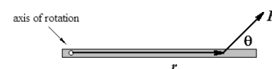
Figure 8.3: A force applied at a point located at \mathbf{r} from the axis of rotation produces a torque \boldsymbol{\tau} = \mathbf{r} \times \mathbf{F} with respect to the axis.
