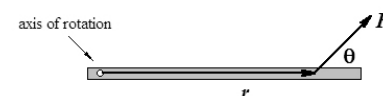
Figure 8.3: A force applied at a point located at \mathbf{r} from the axis of rotation produces a torque \boldsymbol{\tau} = \mathbf{r} \times \mathbf{F} with respect to the axis.
