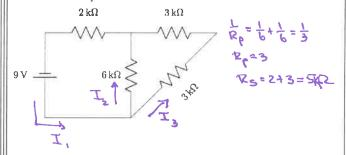
ii. Find the currents across the 2  $k\Omega$  and 6  $k\Omega$  resistors.
