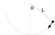
Fig. 3.11. A simple pendulum consists of a point mass m attached to a string of length L . It is released from an angle \theta_0 .
