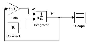
Figure 2.1: Simulink model for exponential growth and decay. The initial value, P(0) = 10, is set in the **Constant** block and k = -0.5 is set in the **Gain**.
