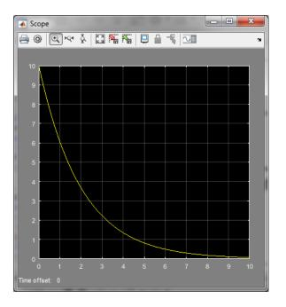
Figure 2.2: Solution for the exponential decay with P(0) = 10 and k = -0.5. The simulation time was set at 10.
