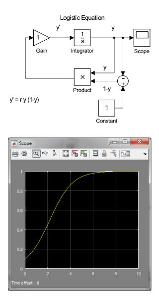
Figure 2.14: Simulink model for the logistic equation, y' = ry(1 - y).
