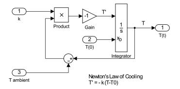
Figure 2.5: Creating a subsystem for the Newton's Law of Cooling model.
