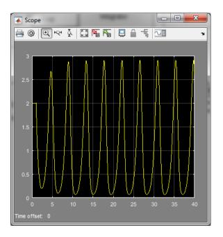
Figure 2.17: Solution of the logistic equation with delay, y' = ry(t)(1 - y(t-1)) for y = 2,  $t \in [0, 1]$ .
