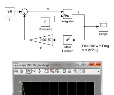
Figure 2.10: Solution for free fall with drag with k = 0.00159 starting from rest.
