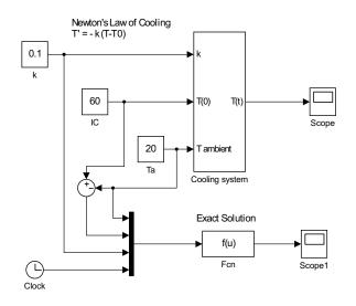
Figure 2.8: Model of Newton's Law of Cooling,  $T' = -k(T - T_a)$ , T(0) = T0, using the subsystem feature.
