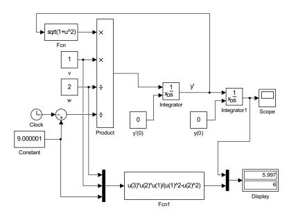
Figure 2.12: Model for the pursuit curve,  $(a - x)y'' = \frac{v}{w}\sqrt{1 + [y'(x)]^2}$ , y(0) = 0, y'(0) = 0, for w = 2 and v = 1.
