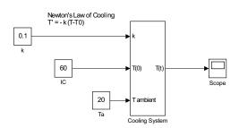
Figure 2.7: Using a user-created subsystem for Newton's Law of Cooling.
