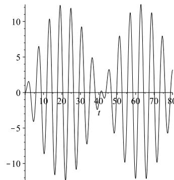
Figure 2.18: Plot of  $x(t) = \frac{800}{129} \left( \cos t - \cos \frac{23}{20}t \right)$ , a solution of  $\ddot{x} + x = 2 \cos 1.15t$ .
