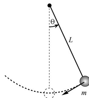
Figure 2.2: A simple pendulum consists of a point mass  $m$  attached to a string of length  $L$ . It is released from an angle  $\theta_0$ .
