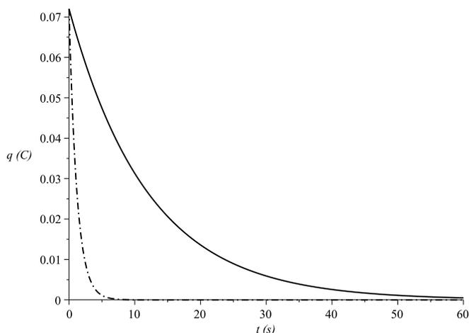
Figure 2.10: The charge as a function of time for a discharging capacitor with  $R = 2.00 \text{ k}\Omega$  (solid) or  $R = 200 \Omega$  (dashed), and  $C = 6.00 \text{ mF}$ , and  $q_0 = 0.072 \text{ C}$ .
