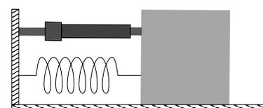
Figure 2.12: A spring-mass-damper system has a damper added which can absorb some of the energy of the oscillations and is modeled with a term proportional to the velocity.
