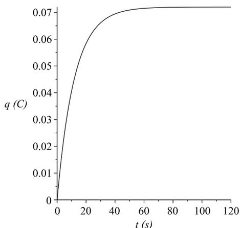
Let's put in some values for the parameters. We let  $R = 2.00 \text{ k}\Omega$ ,  $C = 6.00 \text{ mF}$ , and  $V_0 = 12 \text{ V}$ . A plot of the solution is given in Figure 2.7. We see that the charge builds up to the value of  $CV_0 = 0.072 \text{ C}$ . If we use a smaller resistance,  $R = 200 \Omega$ , we see in Figure 2.8 that the capacitor charges to the same value, but much faster.
