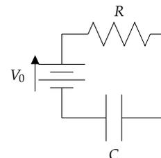
Figure 2.6:  $RC$  Circuit for charging.
