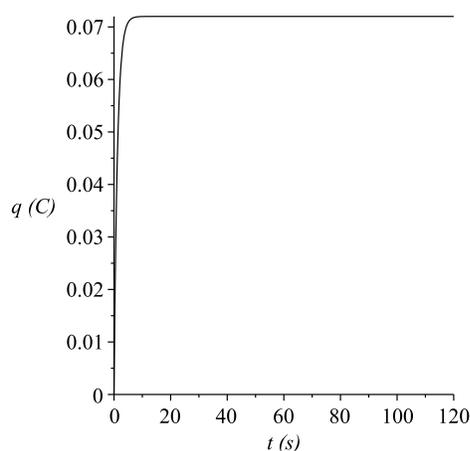
Figure 2.8: The charge as a function of time for a charging capacitor with  $R = 200 \Omega$ ,  $C = 6.00 \text{ mF}$ , and  $V_0 = 12 \text{ V}$ .
