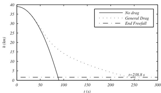
Figure 3.25: Free fall from 39 km at constant  $g$  as compared to nonconstant  $g$  and nonconstant atmospheric density with drag coefficient  $C = .42$ .
