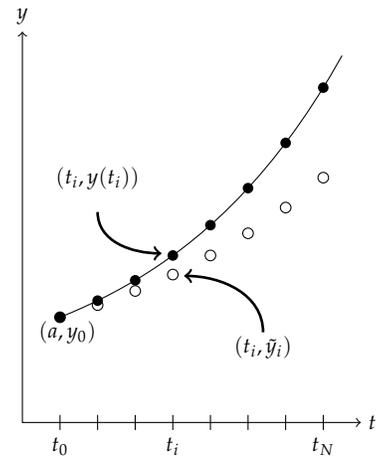
Figure 3.17: The interval  $[a, b]$  is divided into  $N$  equally spaced subintervals. The exact solution  $y(t_i)$  is shown with the numerical solution,  $\tilde{y}_i$  with  $t_i = a + ih$ ,  $i = 0, 1, \dots, N$ .
