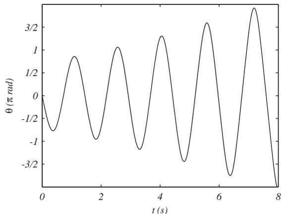
In Figure 3.19 we plot the solution for a starting position of  $30^\circ$  with  $N = 500$ . Notice that the amplitude of oscillation is increasing, contrary to our experience. So, we increase  $N$  and see if that helps. In Figure 3.20 we show the results for  $N = 500, 1000$ , and  $2000$  points, or  $h = 0.016, 0.008$ , and  $0.004$ , respectively. We note that the amplitude is not increasing as much.
