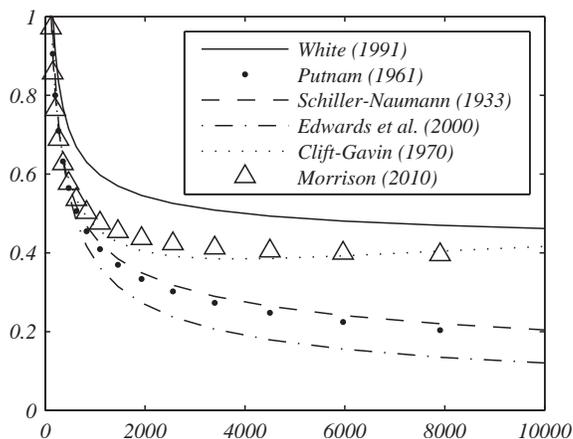
Figure 3.42: Log-log plot of the drag coefficient as a function of Reynolds number for spheres.
