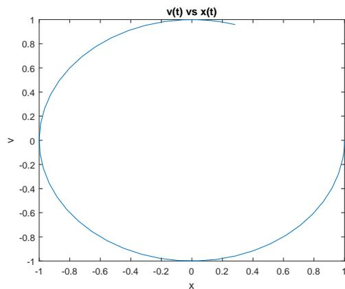
Finally, we can plot a direction field using a quiver plot and add solution curves using `ode45`. The direction field is given for  $\omega = 1$  by  $dx=y$  and  $dy=-x$ .
