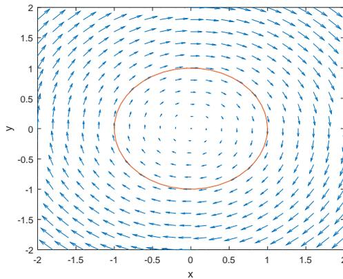
Figure 3.10: Phase plot for the simple harmonic oscillator.
