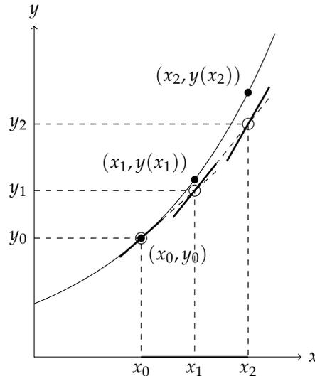
The first step of Euler's Method is to use the initial condition. We represent this as a point on the solution curve,  $(x_0, y(x_0)) = (x_0, y_0)$ , as shown in Figure 3.1. The next step is to develop a method for obtaining approximations to the solution for the other  $x_n$ 's.
