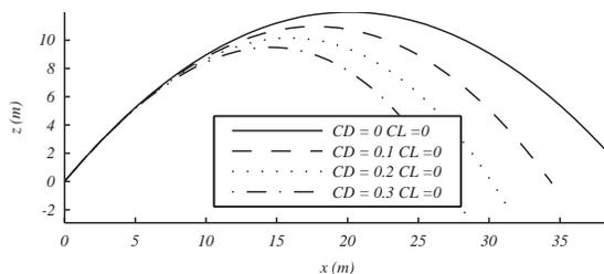
In Figures 3.28 and 3.29 we indicate what typical solutions would look like for different values of drag and lift coefficients. In the case of nonzero lift coefficients, we indicate positive and negative values leading to flight with top spin,  $C_L < 0$ , or bottom spin,  $C_L > 0$ .
