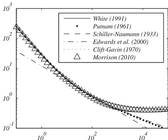
Figure 3.43: A power law fit for the drag coefficient as a function of Reynolds number using linearization and linear regression.
