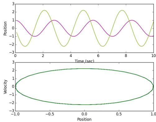
Figure 3.13: Numerical solution of the simple harmonic oscillator using Python's ode routine. In these plots are the position and velocity vs times plots and a phase plot.
