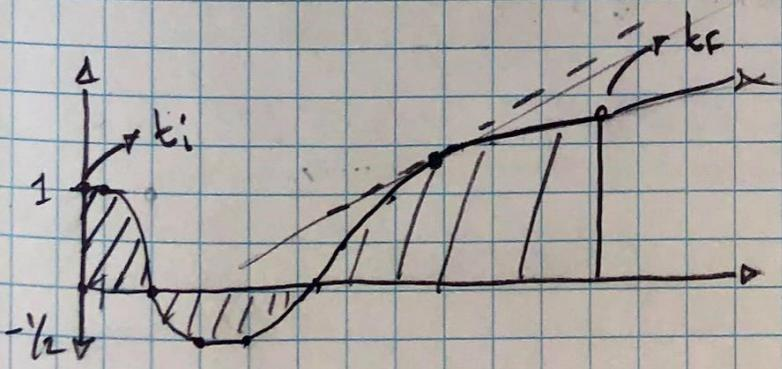
$$x_f - x_i = \text{area under curve } v(t) \text{ from } t_i \text{ to } t_f$$
