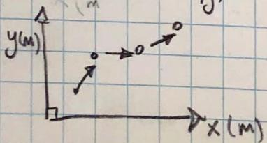
$$\left. \begin{aligned} v_x &= \frac{\Delta x}{\Delta t} \\ v_y &= \frac{\Delta y}{\Delta t} \end{aligned} \right\} |v| = \sqrt{v_x^2 + v_y^2}$$
