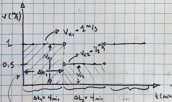
$$\Delta x_1 = v_{x1} \cdot \Delta t_1 = (\text{base}) \times (\text{height}) = \text{area under curve}$$
