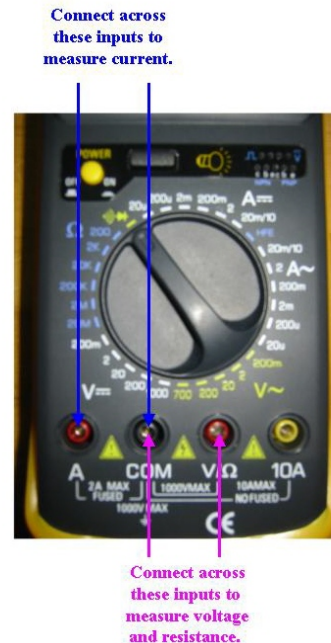
Fig. 2: multimeter input connections
