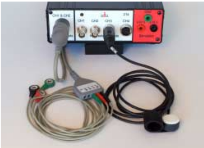
Figure HN-2-5: The EMG cable and pulse transducer connected to an IWX/214.
