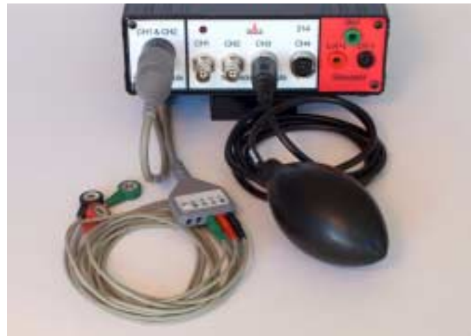
Figure HM-1-3: The EMG cable and hand dynamometer connected to an IWX/214
